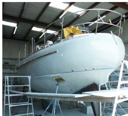
The skag and rudder just attached to the 42'
