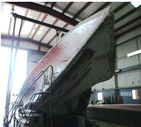
A 50' hull, almost ready to come out of the mold
